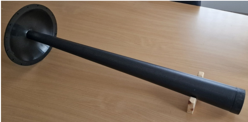
Figure 7: Prototype of the STS section of the CBM vacuum beam pipe. It was produced according to the dimensions of the re-designed STS and manufactured in industry.
