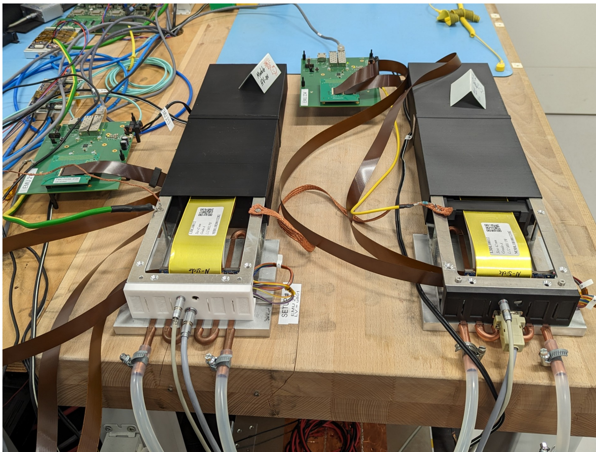
Figure 9. The GBTxEMU boards used for testing the STS detector modules in GSI.
