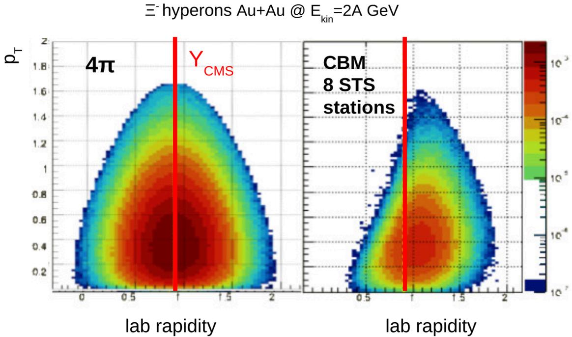
*Fig. 2.2c: Full kinematic phase space (left) and CBM acceptance (right) for  $\Xi^-$  baryons using the new STS geometry design developed in WP2.1.*
