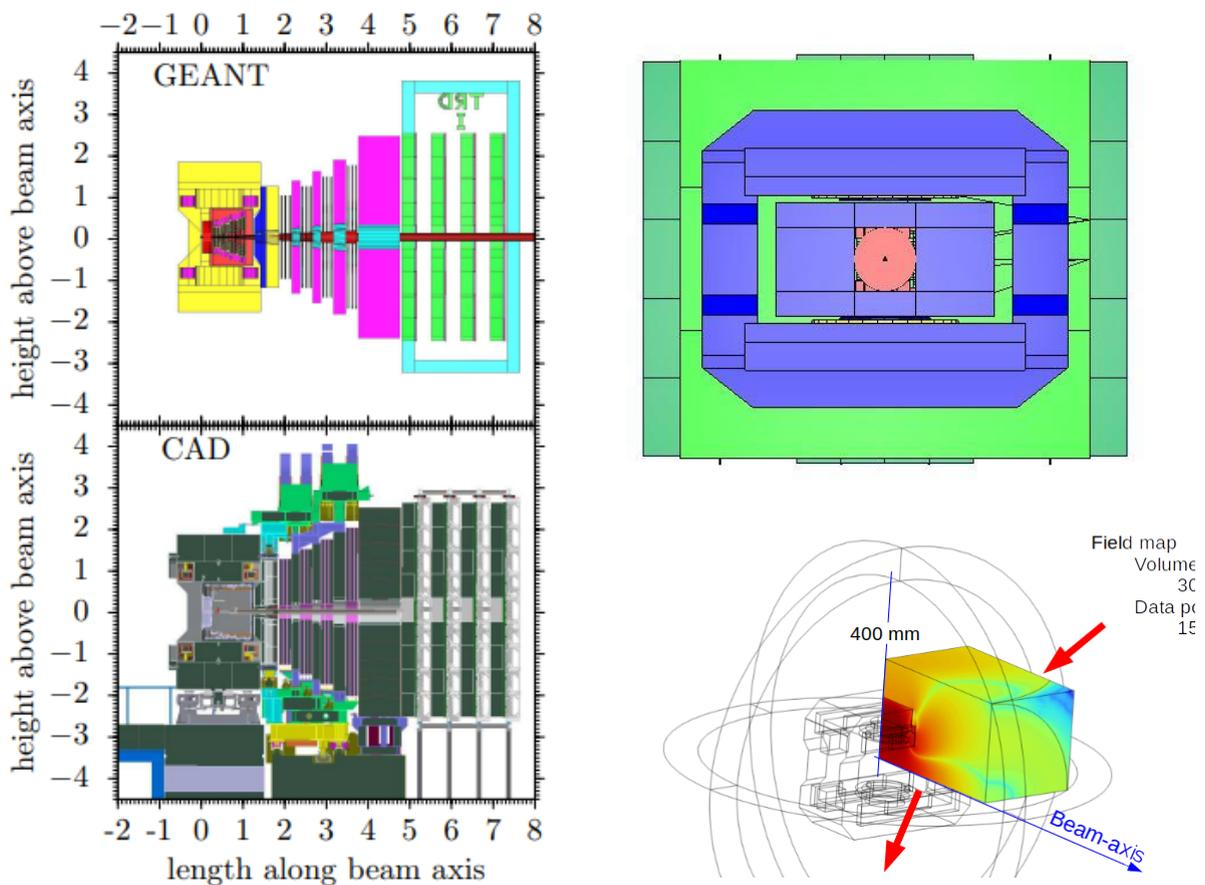
*Fig. 2.2b: CBM geometry as implemented in the (upper left) the GEANT framework used for physics performance studies with Monte-Carlo simulations and (lower left) engineering CAD model (upper left). New (upper right) magnet geometry and (lower right) magnetic field map.*
