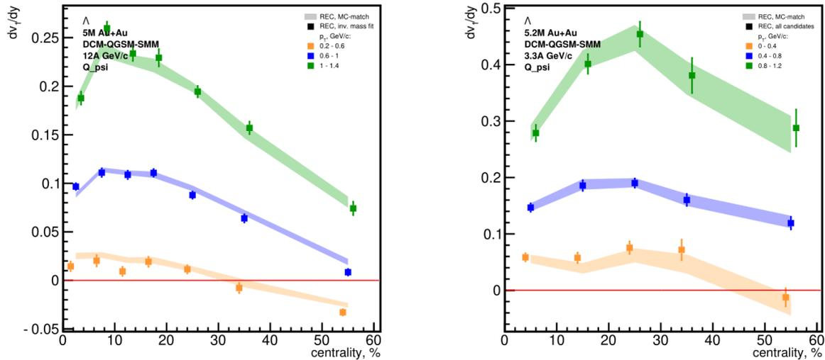
Fig. 2.4b CBM performance for directed flow measurement of  $\Lambda$  hyperons as a function of centrality highest (4.9 GeV) and lowest (2.9 GeV) collision energies of SIS-100 accelerator at FAIR.
