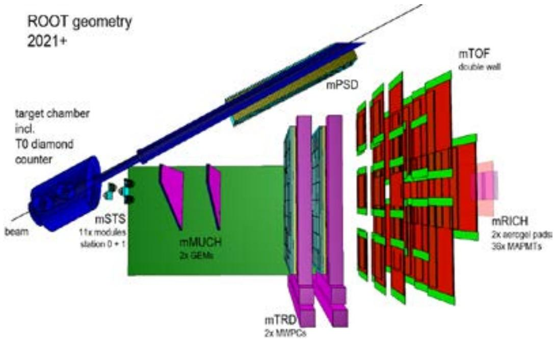
*Fig. 2.1a Geometry of the mCBM experiment as implemented in the GEANT simulations.*
