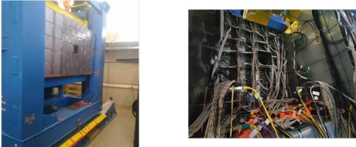
Fig. 3: Left: Photo of the FHCAL front view installed at the BM@N experiment. Right: Rear view of the calorimeter with installed FEE and readout electronics.
