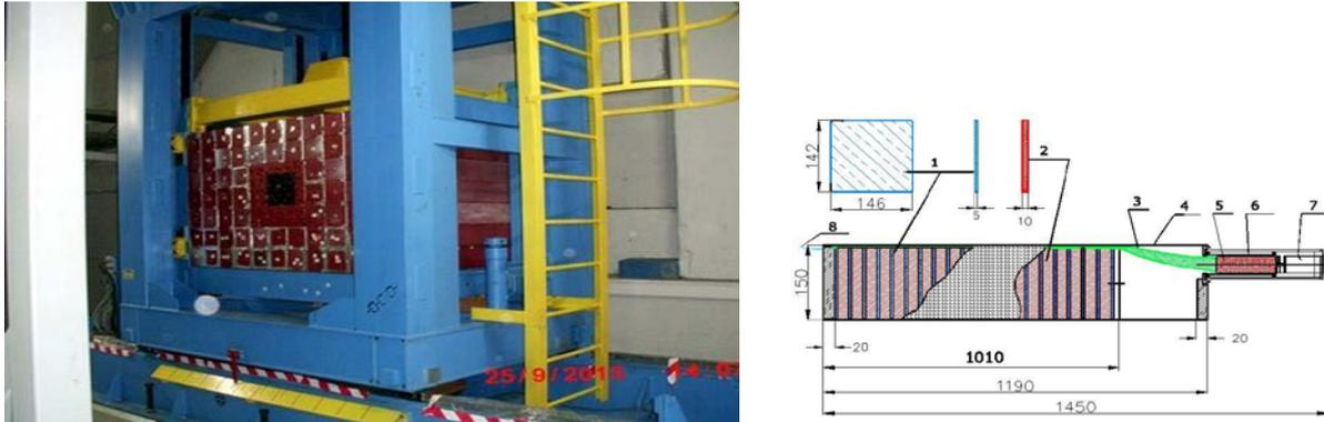
Fig. 1: Left: Photo of the BM@N ZDC. Right: Schematic view of the ZDC module (details see in [3]).
