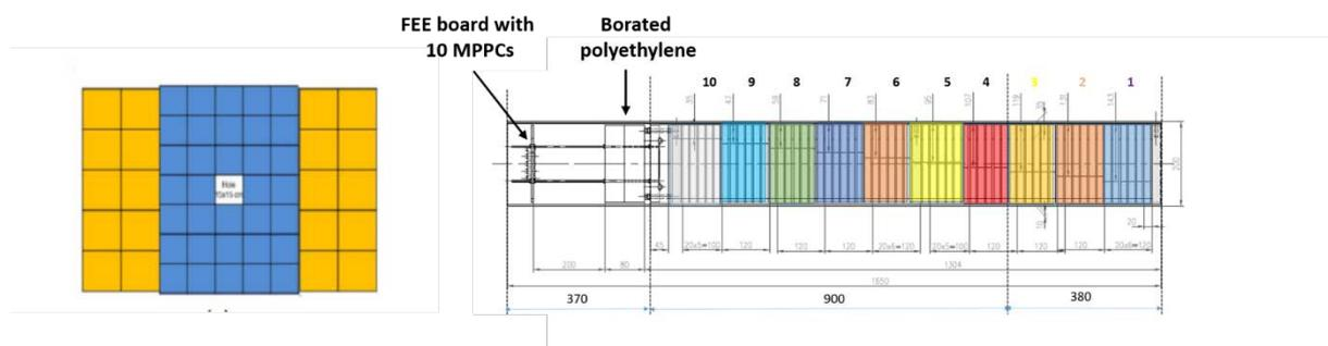
Fig. 2: Left: The scheme of the FHCAL. Right: The scheme of the CBM PSD module used at the FHCAL. The different colors indicate 10 longitudinal sections of the module.
