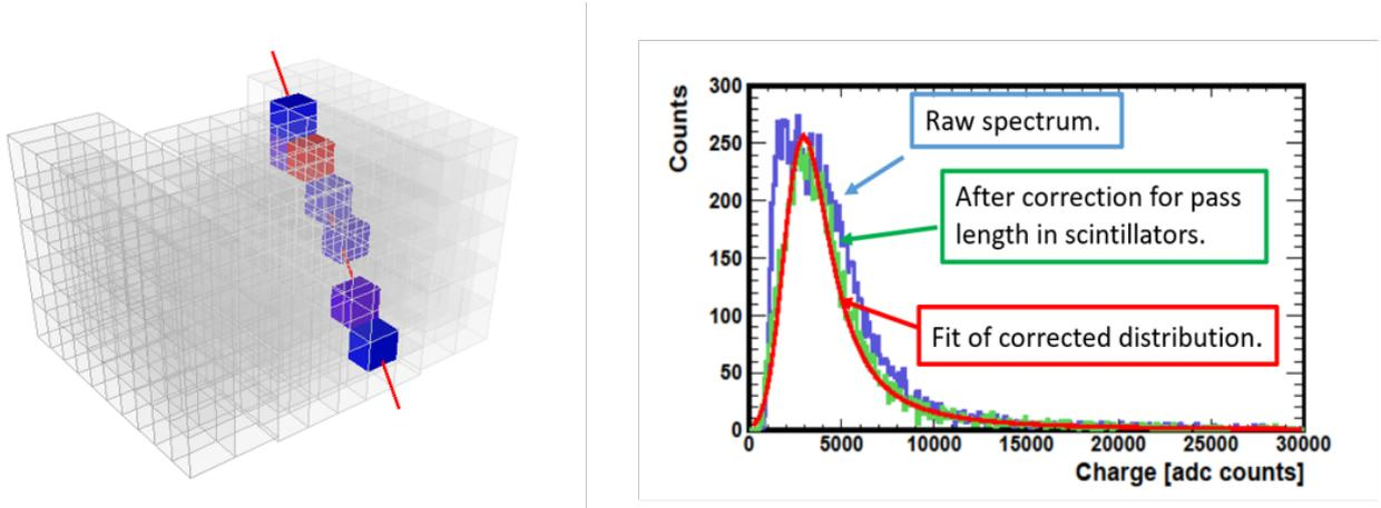
Fig. 4: Left: Sketch of a 3D view of a muon track in the FHCAL. Right: Track length correction in one of the sections of the FHCAL module. Blue curve: Muon spectrum before the correction. Green curve: Muon spectrum after the correction of the track length. Red curve: Corrected muon spectrum fitted by a Landau and a Gaussian function (langaus).
