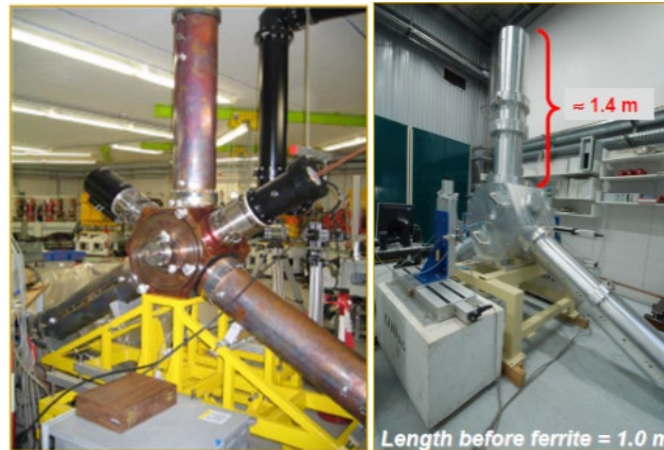
Figure 7-10: Accelerating cavity of the BESSY accelerator (left) and ESRF (right).
