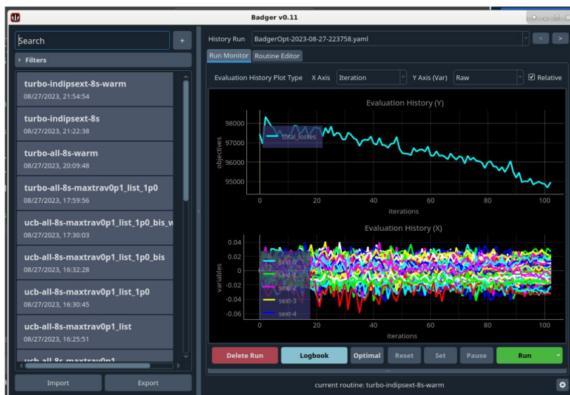
Figure 16: Badger application run monitor panel. The objective of minimization is displayed in the top plot, while the relative change of the parameters used for tuning is presented in the bottom plot. Users can easily customize the plotting preferences at any time through the toolbar, including options like using time as the x-axis instead of the iteration index or displaying normalized values of the variables.
