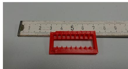
Figure 14: Sample holder for nine powder-filled capillaries for *ex-situ* XAS measurements [2].
