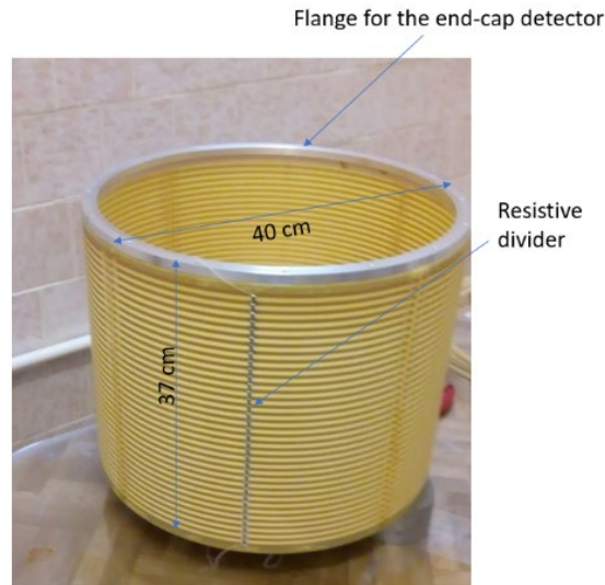
Figure 10. Assembled field cage with the fixation ring glued and resistive divider mounted.
