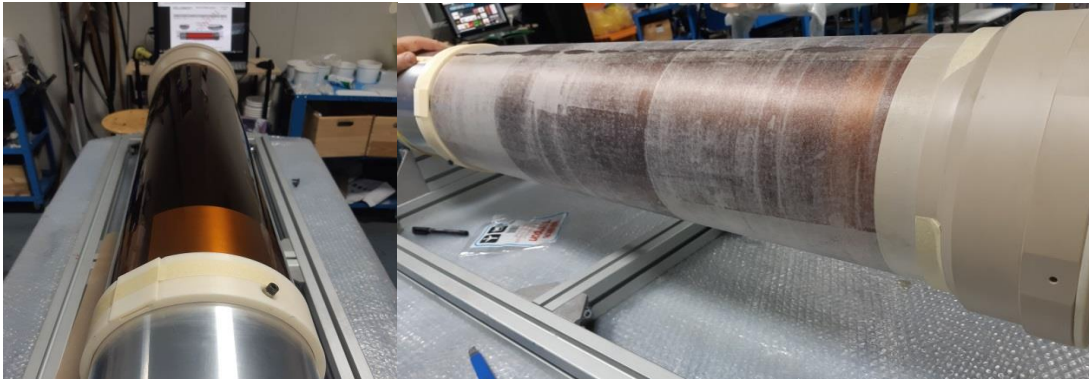
Figure 19. Cathode lamination: the initial copper layer (left) and the fiberglass deposition (right).
