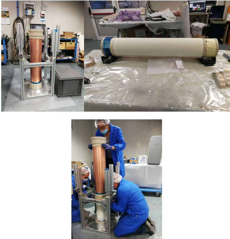
Figure 26. Assembly of the prototype. From top left: the cathode mounted on the assembly machine; the rectified Millifoam support for the detector tiles; the insertion of the cathode on the cylindrical anode.
