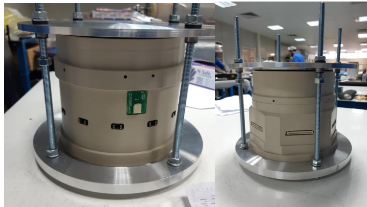
Figure 25. Setup for the gas tightness tests of the HV flange (left) and FEE flange (right).
