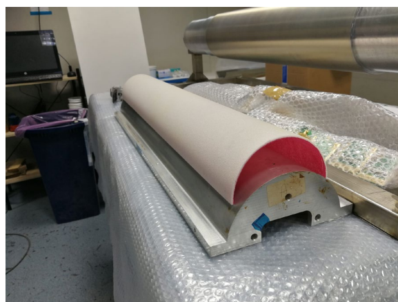
Figure 23. Millifoam support for the tile.
