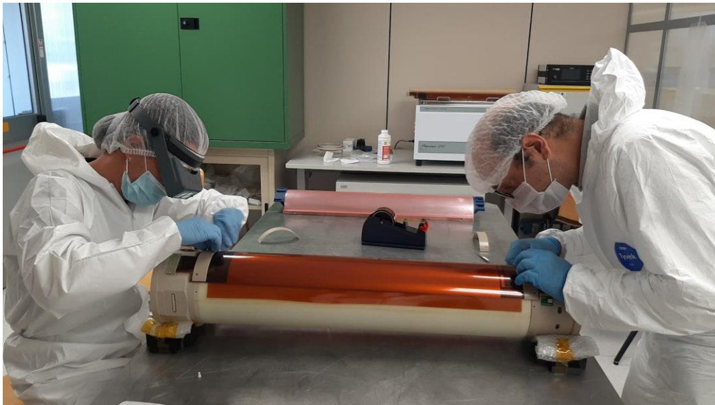
Fig. 3.5: The assembly of an anode roof-tile on the Millifoam structure.
