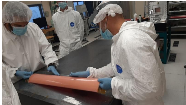
Fig. 3.2: Transfer of the epoxy-glue from the polypropylene foil to the Millifoam roof tile.
