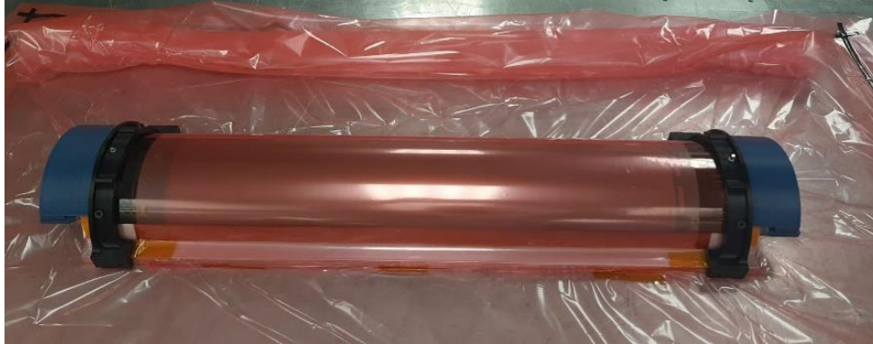
Fig. 3.3: An anode circuit after the glue curing cycle. Counter-flanges at the edges are visible in this picture (black and blue).
