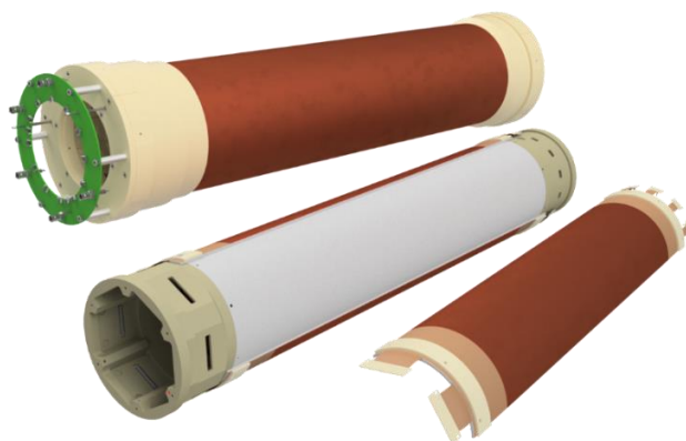
Fig. 2.5: Sketch of the assembly of the three roof-tile detectors on the anode cylinder. The anode cylinder is made of composite material: FR4 - Millifoam - FR4 sandwich plus an additional finely machined layer of Millifoam.
