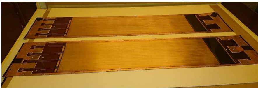
Fig. 2.6: Flexible \mu -RWELL_PCB detector tiles manufactured at the CERN MPT Workshop.
