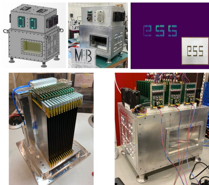
1. Figure 1: Multi-Blade TBL detector, as constructed for operation on the TBL, clock-wise: CAD-model, bare vessel, ESS mask reproduced with neutrons, internal 14 units mechanics, the whole detector with electronics but without electronics box.
